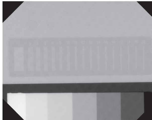
Fig. 11. Radiographic image of dental digital quality assurance phantom on defective sensor.
